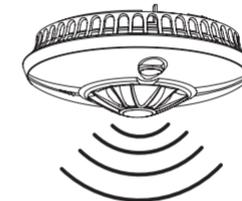
6. PLEASE NOTE: If the test button is not pressed quickly enough (before the red LED on 'Alarm 2' has gone out), the 'learn-in' process will fail. If this happens, repeat the process again, as described above.
