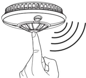
2. The unit will give an audible alarm consisting of 2 cycles of 3 loud beeps, then stop automatically.
